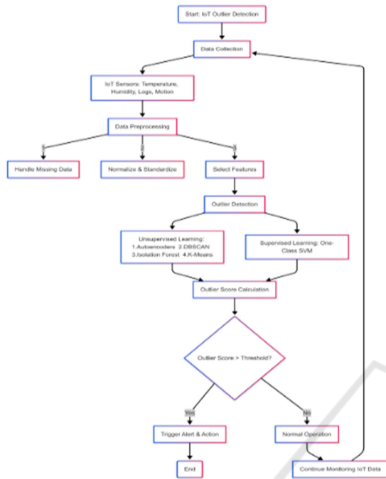
Figure 1: Architecture of Outlier Detection System.
