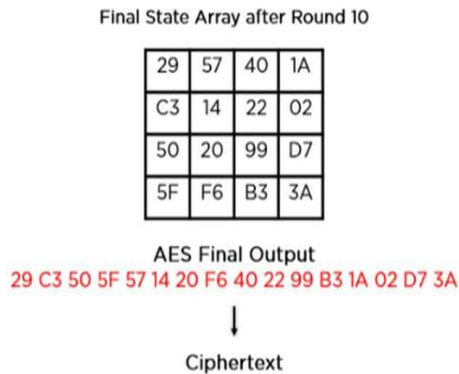
Figure 14: Final State Array and Ciphertext Output After 10 Rounds of AES.
