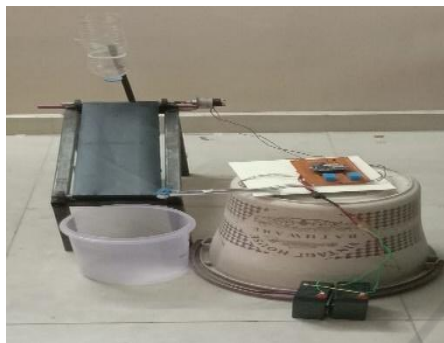
Figure 4: Prototype of Automated in Level Detection and Conveyor Control System for Polymer Manufacturing.
