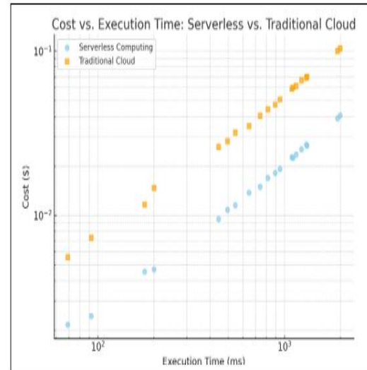
Figure 3: Cost Efficiency in Serverless Computing Vs. Traditional Cloud Models.
