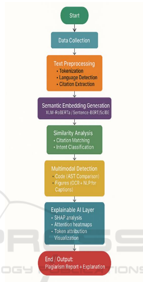
Figure 1: Workflow of the Proposed Plagiarism Detection Framework.
