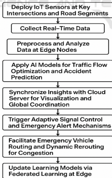
Figure 1: Workflow of the IoT-based intelligent transportation and accident management system.
