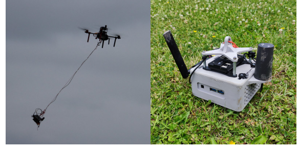
(a) Photo from experiment (b) Payload with RTK GNSS Figure 7: Experimental hardware used in the field deployment.
