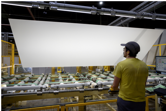
Figure 4: Manual quality inspection of decorative surfaced panels at Sonae Arauco's factory (Ricardo Castelo, 2024).
