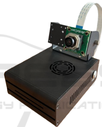
Figure 5: Image acquisition system featuring an NVIDIA Jetson Nano in an industrial enclosure, paired with an RGB camera.
