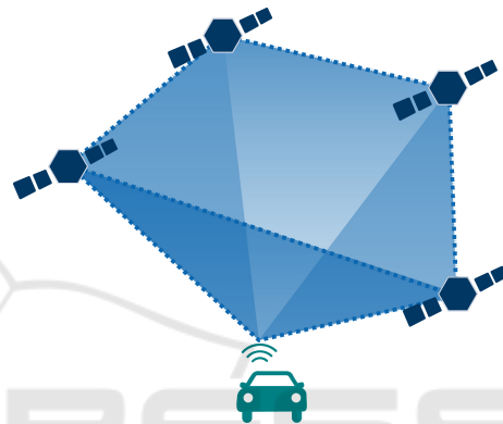
Figure 1: Visualisation of geometry for the PDOP between receiver and satellites.
