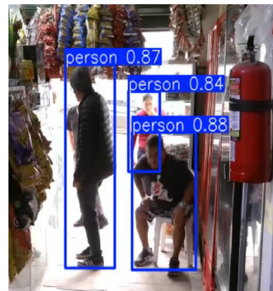
Figure 1: the system identifies customers upon entry and tracks their interaction with products.
