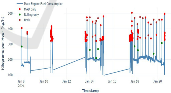
Figure 3: Outlier detection using a hybrid method on main engine fuel consumption.
