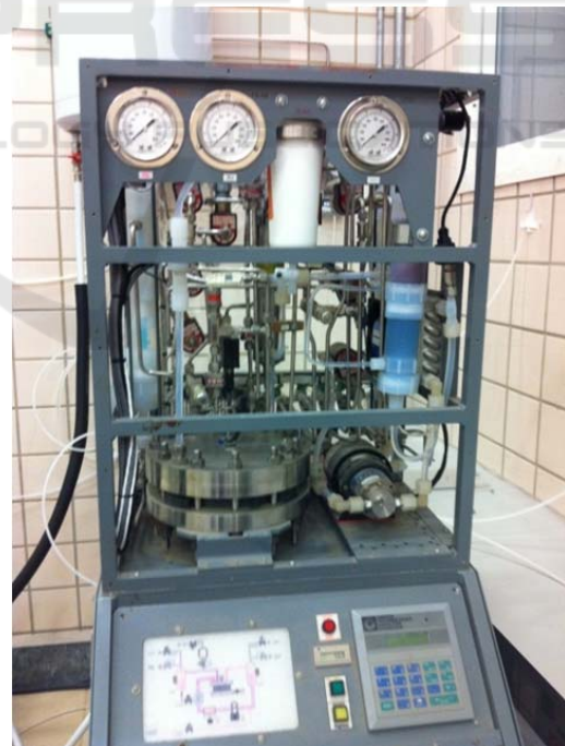
Figure 1: Front view of the PEM Electrolyzer.
