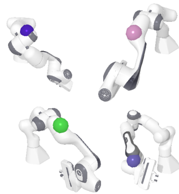
Figure 2: Four rendered frames from the contact experiments. In each run, the Franka Emika robot is tasked with making contact with a specific point inside its task space (a small, colored sphere is used to represent said point) but has only a set amount of C-space moves to get there. It is observed and validated that contact is apparently achieved.
