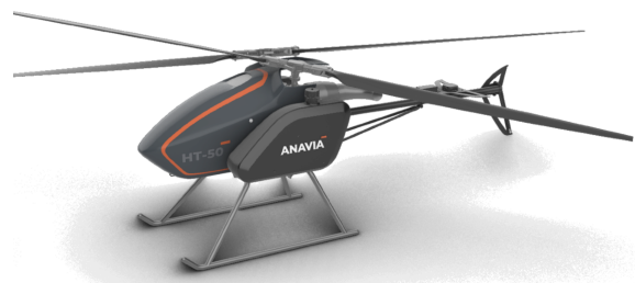
Figure 3: HT-50 from ANAVIA was developed as a training platform for the larger HT-100. It has a payload of 20 kg, a flight time of 90 min and a maximum speed of 100 km/h.
