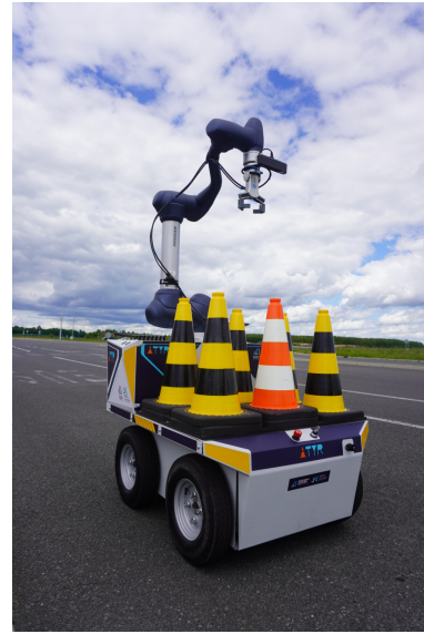
Figure 2: Heavy duty robot platform for traffic cone manipulation.
