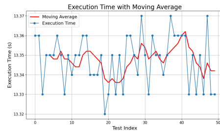
Figure 6: Execution time per cycle for 50 trials, with the moving average in red.
