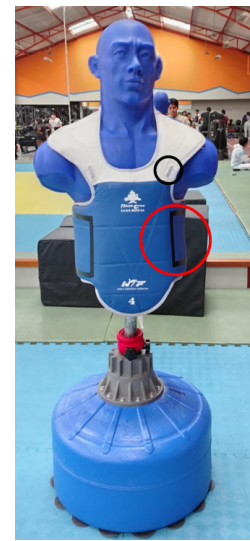
Figure 3: Location of the components on the chest protector. Red circles indicate the position of the piezoresistive sensors, while black circles indicate the placement of the LED strips for visual stimulation.
