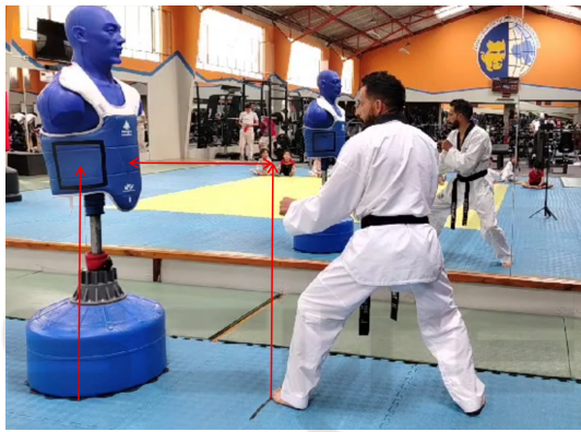
Figure 4: Experimental setup configuration for testing the instrumented chest protector. Red lines indicate participant-specific distance adjustments made to ensure proper alignment and comfort.
