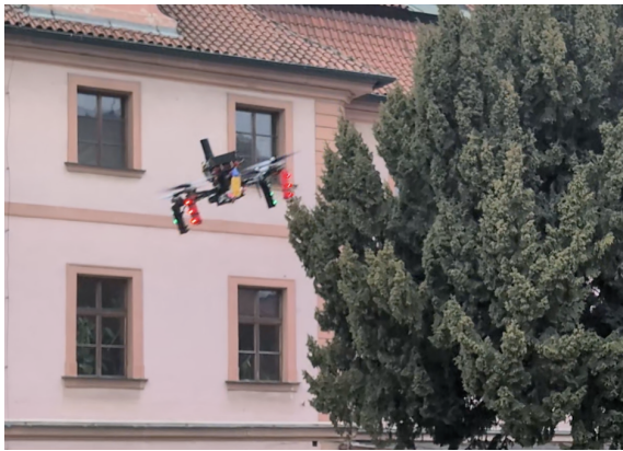
Figure 1: Illustration from real-world flight: quadrotor in flight using proposed learned policy.
