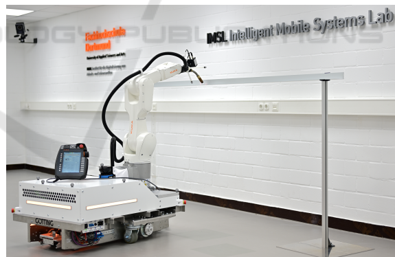
Figure 1: MobileRobot: Omnidirectional mobile platform with a 6-DoF manipulator.
