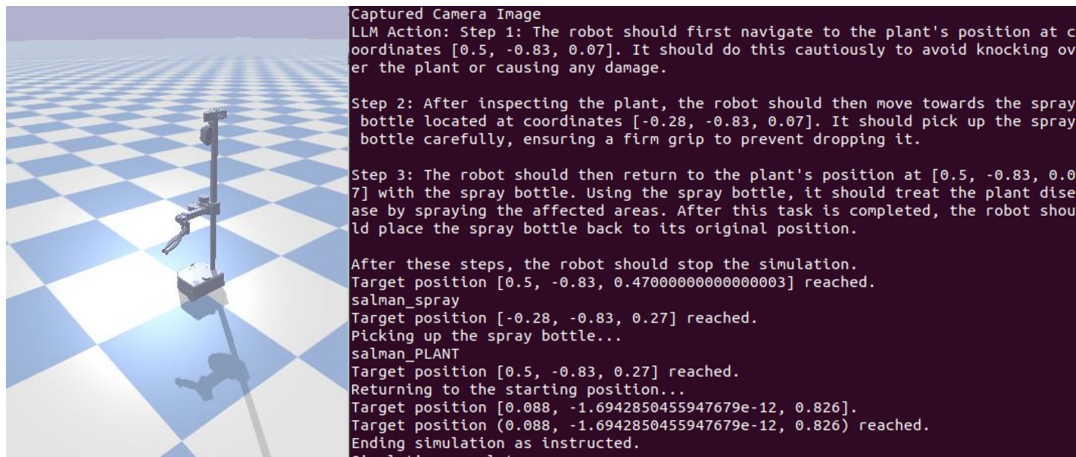
Figure 10: Implementation of LLM based planning with low level control based on perception input in simulation environment.
