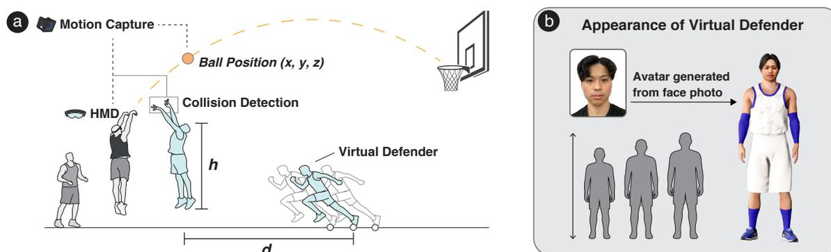
Figure 1: Overview of the proposed system and virtual defender. (a) Real-time motion capture and collision detection for simulating defensive pressure in MR. (b) Virtual defender appearance generated from facial photo with adjustable body attributes.
