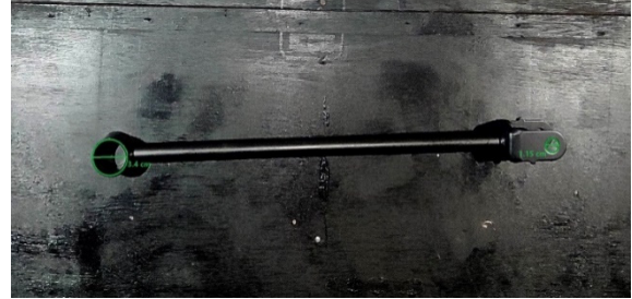
Figure 5: Correctly Detected circle diameter on rod using Proposed Method
