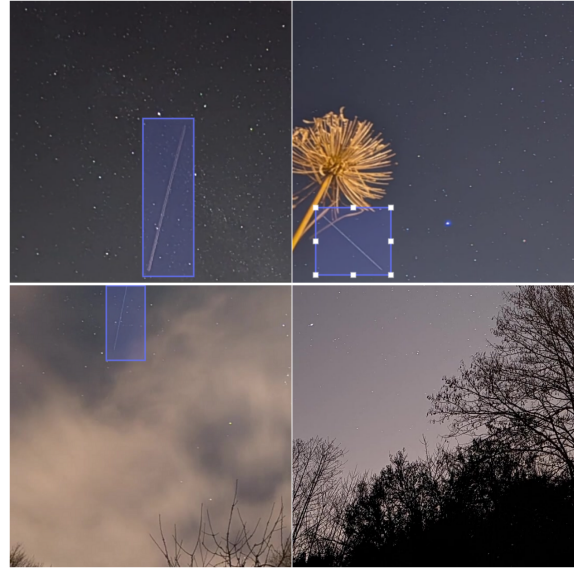
Figure 2: Four 640 \times 640 annotated images in the training set: the last one is for background, i.e. without label, to learn the model to ignore undesired patterns in the image.
