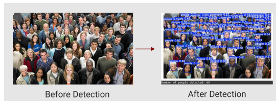
Figure 5: YOLOv10 detecting individuals in a moderately dense crowd, with a total count of 69.
