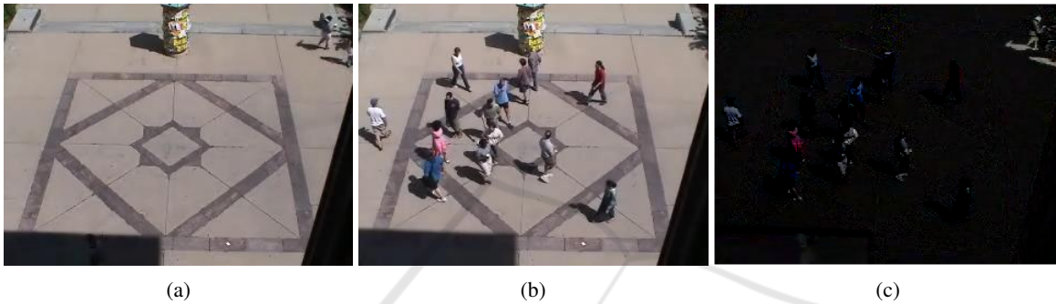
Figure 2: Background Subtraction, a)Background Frame, b)Current Frame, c)Foreground object frame.
