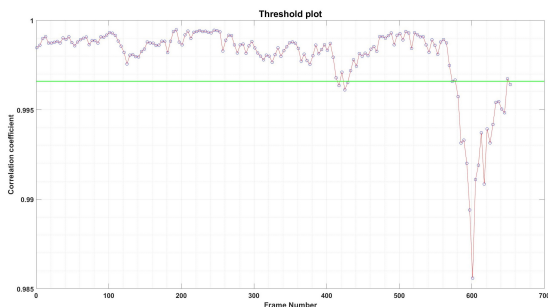
Figure 8: Threshold plot for a video with threshold selected at th=0.9966
