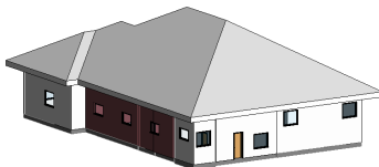
Figure 5: External view of 3D Building Information Modeling (BIM) model of 2D drawing.
