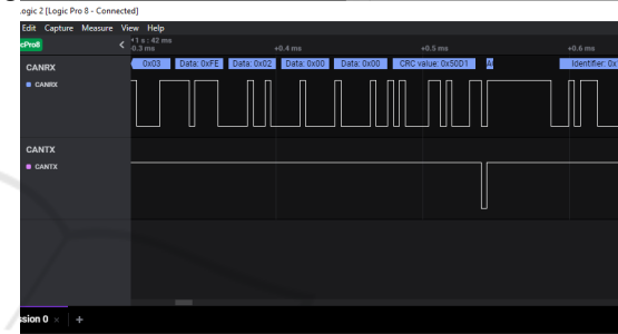
Figure 6: CAN Reception Signal on Logic Analyzer
