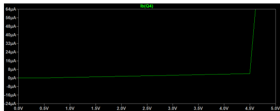
Figure 11: Cell Voltage v/s Base Current
