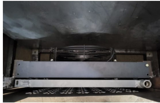
Figure 5: Radiator used for cooling
