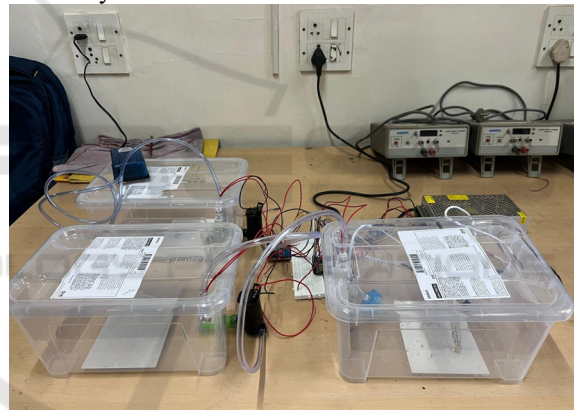
Figure 2: Prototype with Tank 2,3 and 4 where aeration, chlorination, sedimentation, and UV treatment take place.
