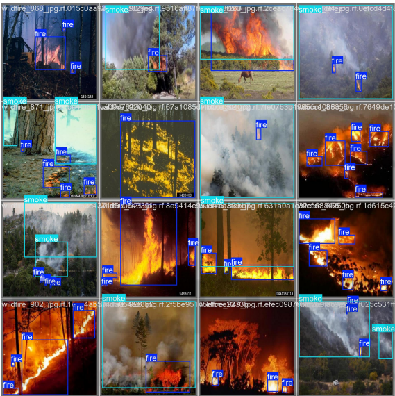
Figure 7: Sample Output of our YOLO11 model identifying smoke and flames in diverse forest conditions. The bounding boxes display the model’s capability to detect small fires and faint smoke effectively.
