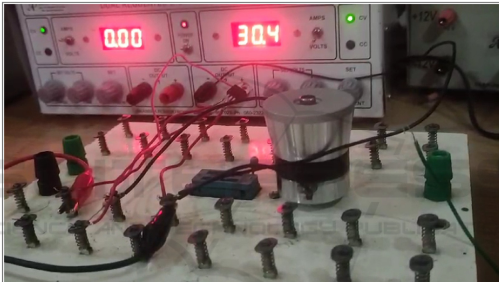
Figure 6: Initial setup with the temporary ultrasonic cleaner transducer.
