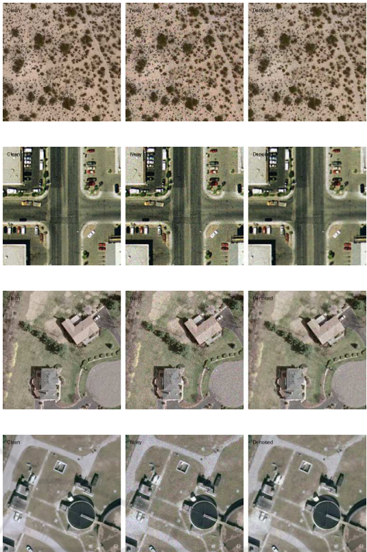
Figure 2: Denoising results for Standard HOTV Model with Speckle Noise. In each figure, the first image is clean, the second is noisy, and the third is restored.
