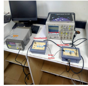
Figure. 6: Experimental Set Up for loss measurement
