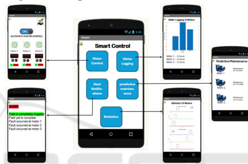
Figure 13: Comprehensive Mobile Application Interface for Smart Irrigation System Management
