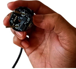
Figure 2: CMOS sensor obtained from a 1600x digital USB microscope.
