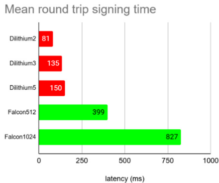
Figure 7: Mean round trip signing times in ms using a linear scale showing Dilithium as the fastest scheme and Falcon being five times slower.
