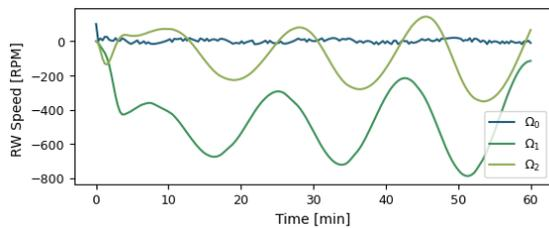
Figure 6: Reaction Wheels speed with PD controller.
