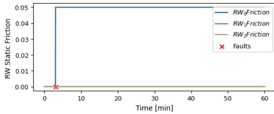
Figure 2: One-time static friction fault.
