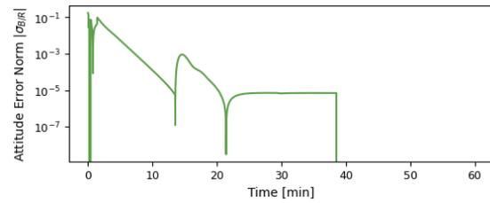
Figure 4: Impact of one-time static friction fault on attitude.
