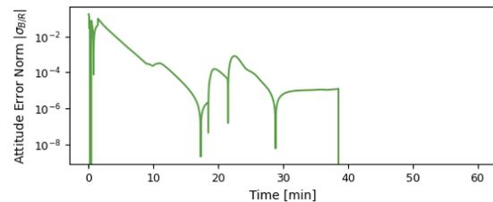
Figure 5: Impact of continuous smaller static friction fault on attitude.
