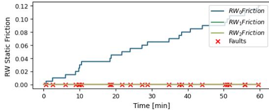
Figure 3: Continuous smaller static friction fault.
