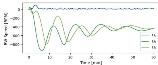
Figure 8: Reaction Wheels speed using magnetic torquers.
