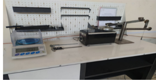
Figure 2: A device with a diamond disc that determines wear resistance.
