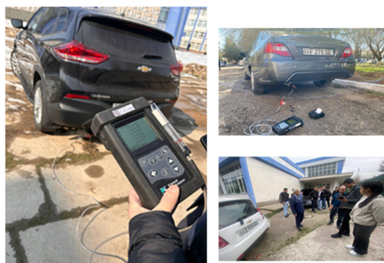
Figure 1: Taking exhaust gas readings from a car engine on the Kane AUTO plus gas analyzer.
