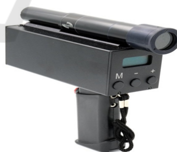
Figure 3: Kelvin PLTs 3000 equipment for measuring the temperature of a liquid alloy (Nodir et al., 2022).
