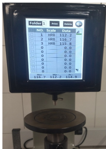
Figure 1: “TP-5018 PAC Tochline” hardness measurement machine.
