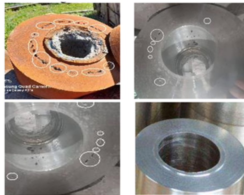
Figure 3: Appearance of gas porosity in cast products.
