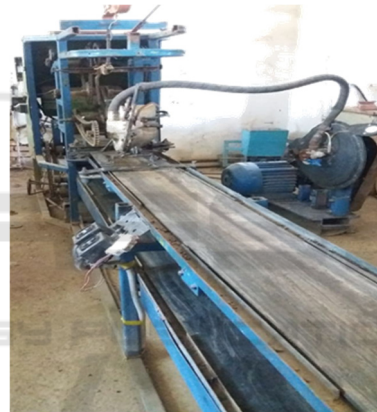
Figure 2: General view of laboratory stand equipped with improved pneumatic planting apparatus.
