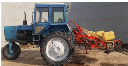
Figure 1: General view of an experimental instance of a pneumatic seeder that precisely seals seeds without feathers into a tractor.
