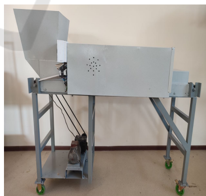
Figure 1: An overview of the first ultra-high-frequency electric magnetic field treatment device for cocoons.
