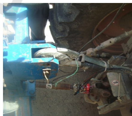
Figure 3: The position of the tension fingers on the device's hinge and cardan.
