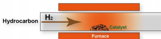
Figure 4: Schematic representation of a CVD apparatus for growing CNTs (Zhao, 2014).
