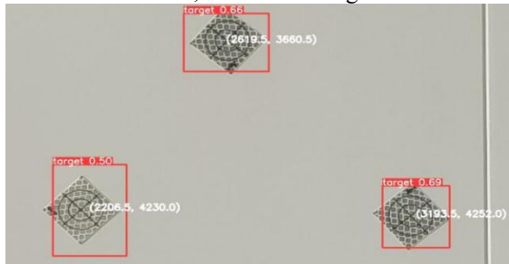
Figure 4: YOLOV5 Target center coordinates acquisition.
