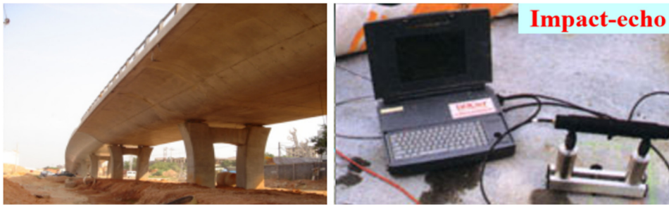
Figure 4: The IE method to detect the grout quality on site.
