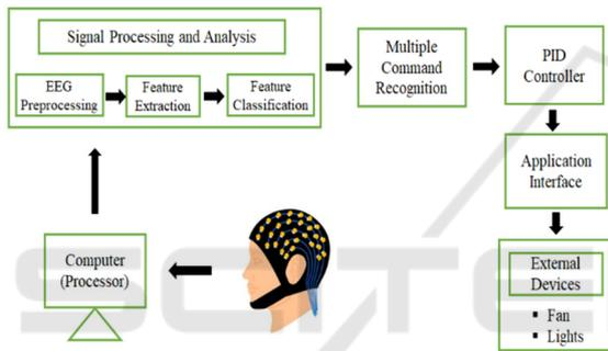
Figure 3: Block Diagram of BCI-Driven Smart Home Automation System.
